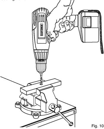
WARNING: Be prepared for binding or bit breakthrough. When these situations occur, drill has a tendency to grab and kick opposite to the direction of rotation and could cause loss of control when breaking through material. If not prepared, this loss of control can result in possible serious injury.
